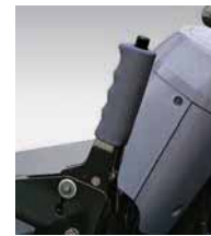
Notch-release parking brake
